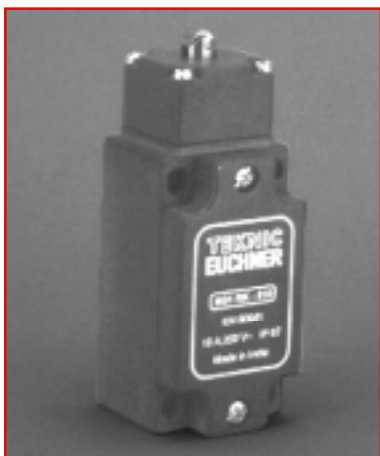
Limit switch with short roller plunger RK. Hardened roller with plain bearing. Operating point reproducibility \pm 0.01 mm. Approach speed max. 50 m/min.
