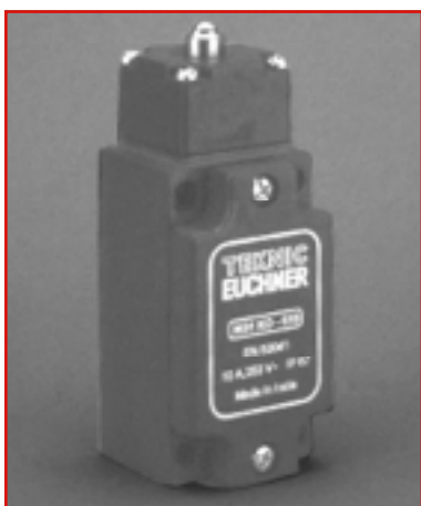
Limit switch with ball plunger KO. Hardened ball can be actuated from various directions. Operating point reproducibility \pm 0.01 mm. Approach speed max. 10 m/min.
