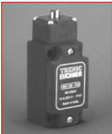
Limit switch with chisel plunger DO. Hardened and polished. Operating point reproducibility \pm 0.002 mm. Approach speed max. 10m/min.
