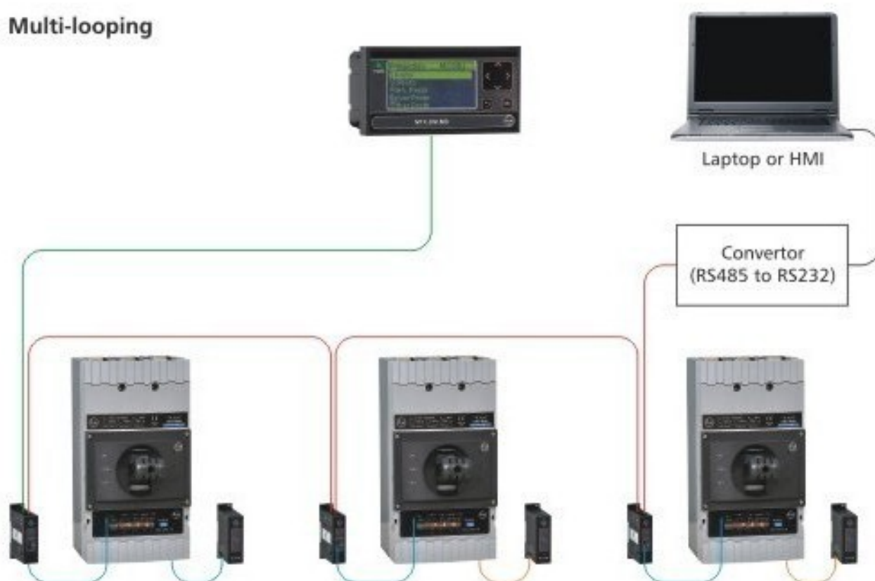
MODBUS Communication through MODBUS looping
